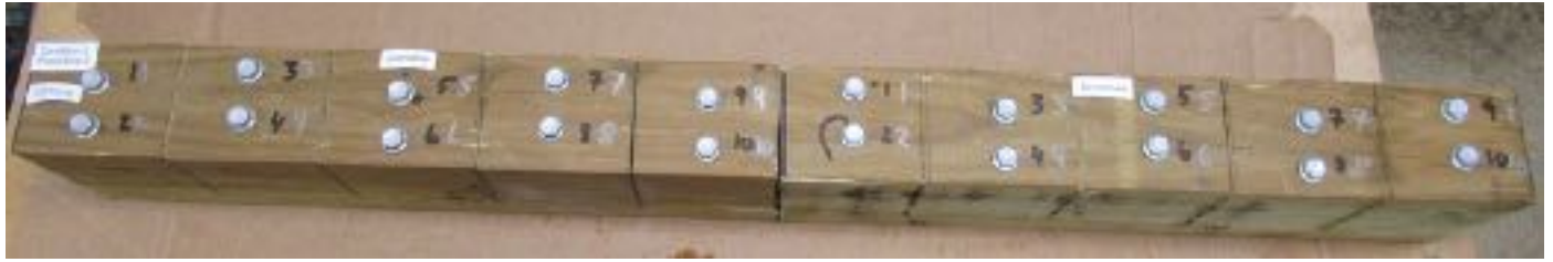
Fasteners, Procedure 2 (G-85), Progressive Head Corrosion 336 hours
