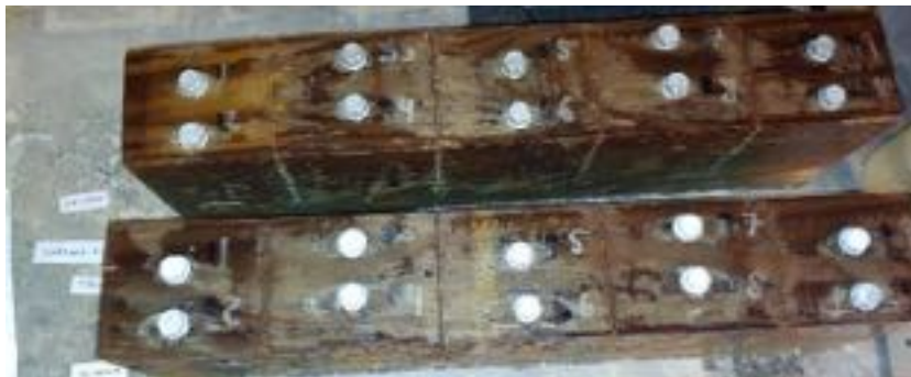
Fasteners, Procedure 1 (B117), Progressive Head Corrosion 1008 hours
