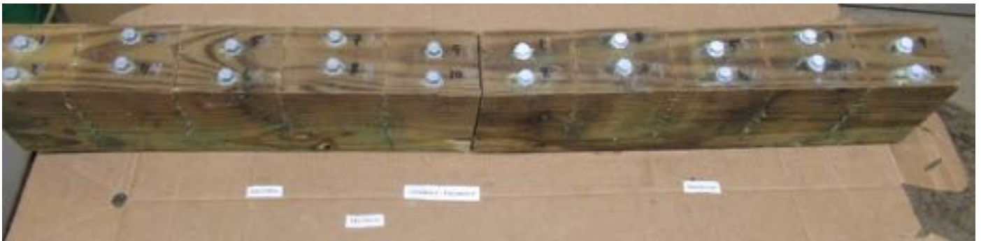
Fasteners, Procedure 1 (B117), Progressive Head Corrosion 1440 hours
