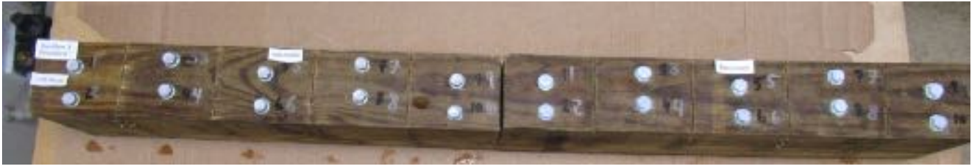
Fasteners, Procedure 1 (B117), Progressive Head Corrosion 336 hours
