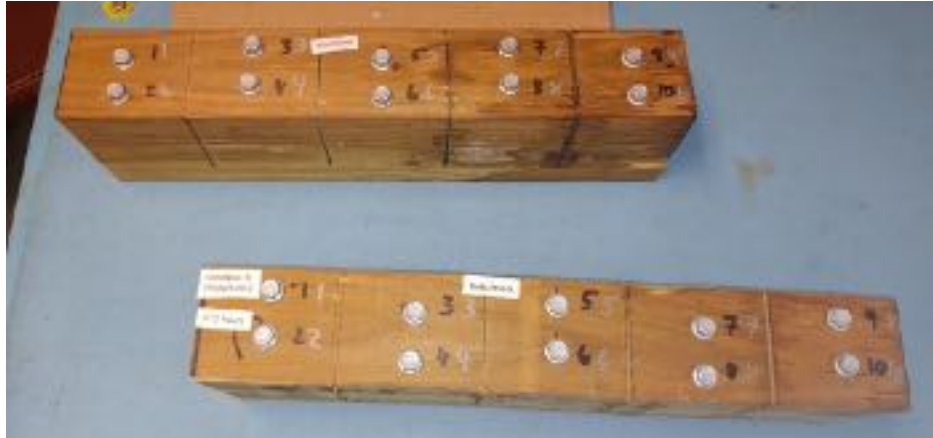
Fasteners, Procedure 2 (G-85), Progressive Head Corrosion 672 hours
