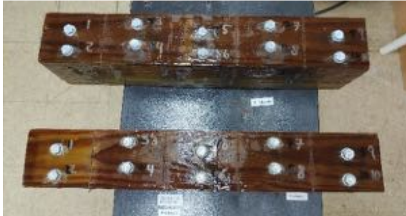
Fasteners, Procedure 1 (B117), Progressive Head Corrosion 672 hours
