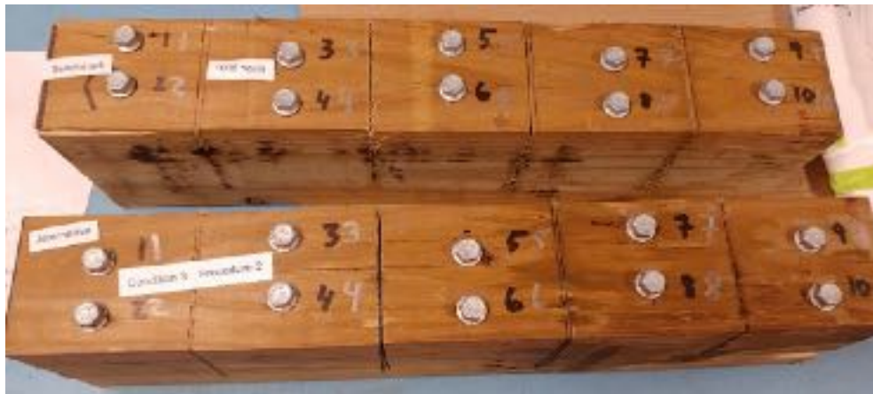
Fasteners, Procedure 2 (G-85), Progressive Head Corrosion 1008 hours
