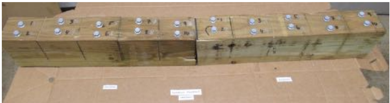
Fasteners, Procedure 2 (G-85), Progressive Head Corrosion 1440 hours
