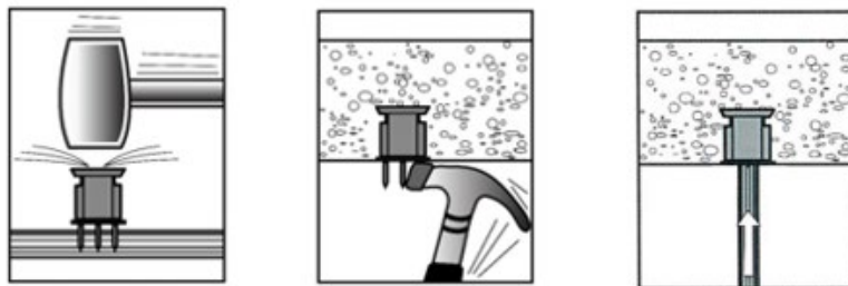
FIGURE 6—PIP INSTALLATION INSTRUCTIONS
